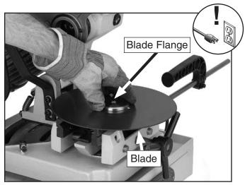
Figure 25. Installing new blade.
